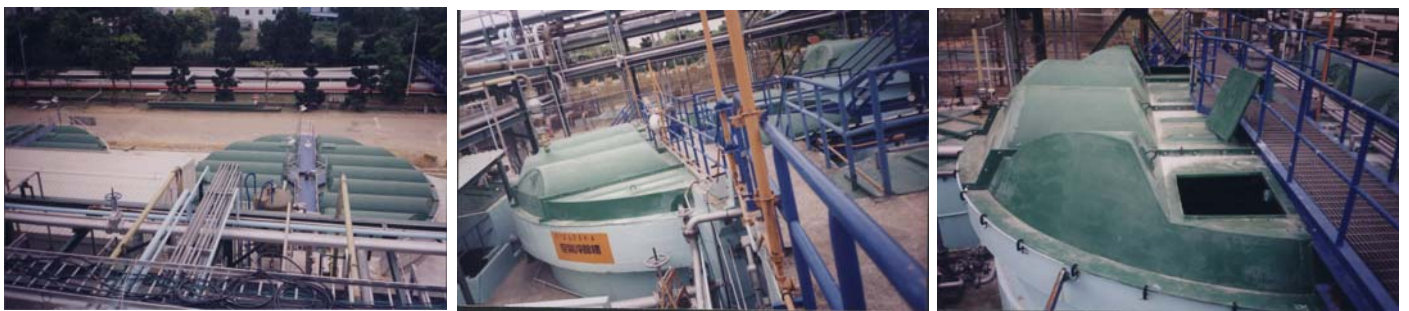
平行拱頂型 (BARREL VAULT ROOF- parallel segmented)
